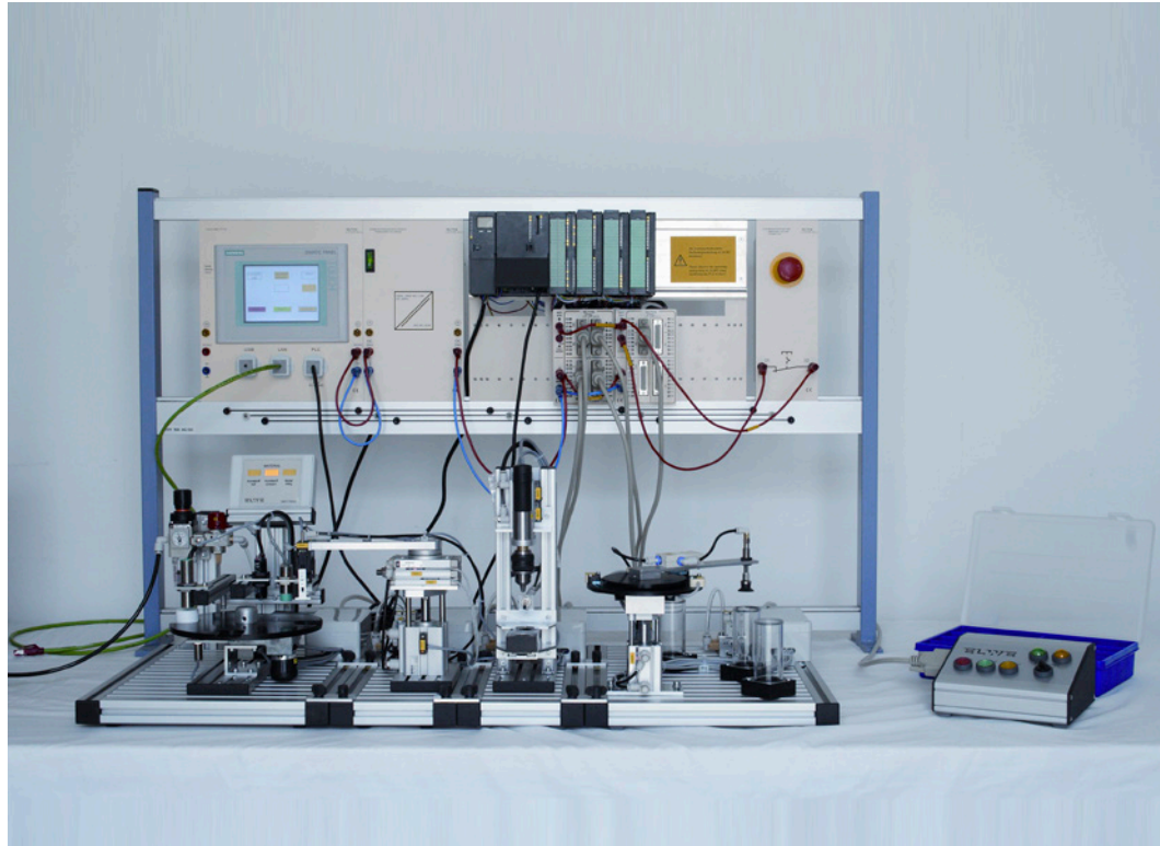
MCS with PLC for 5 Stations (E6.7.2.2)
